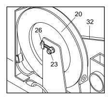
counterclockwise. Make sure that the Flywheel is straight and retighten the M10 Flange Nuts (23). When the Drive Belt is properly adjusted, re-attach the side shields.
